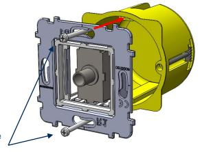
Screws supplied with the flush-mount box.
