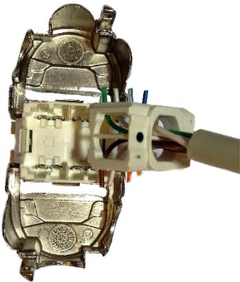
3. Replace the connection block (one way only using the polariser) after making a clean cut on the 8 wires.
