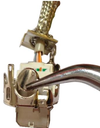
4. Remove the cover to pass the cable through (rear or side), then close the 2 flaps of the RJ45 block.
