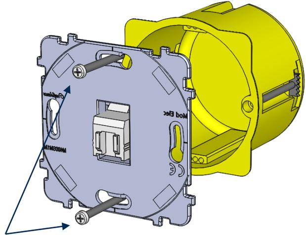
Screws supplied with the flush-mount box.
