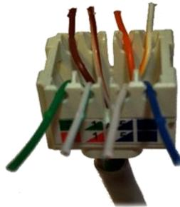
2. Run the wires along the side or rear (as desired), then individually through the notches provided, following the colour code in line 6A.
